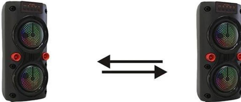
2. Short press "SCAN/II" button on one unit when hear "DIDI", then the two units are connected successfully, and the bluetooth indicate light on one of the unit change to blue.
